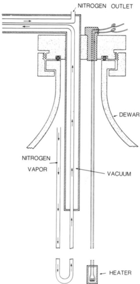
Fig. 2. Internal details of storage Dewar, with nitrogen vapor as coolant (sectional view). The inlet to the coolant tube is located near the top of the Dewar, projecting above the surface of the liquid nitrogen. The "U" turn of the coolant tube and the heater are located near the bottom of the Dewar.
