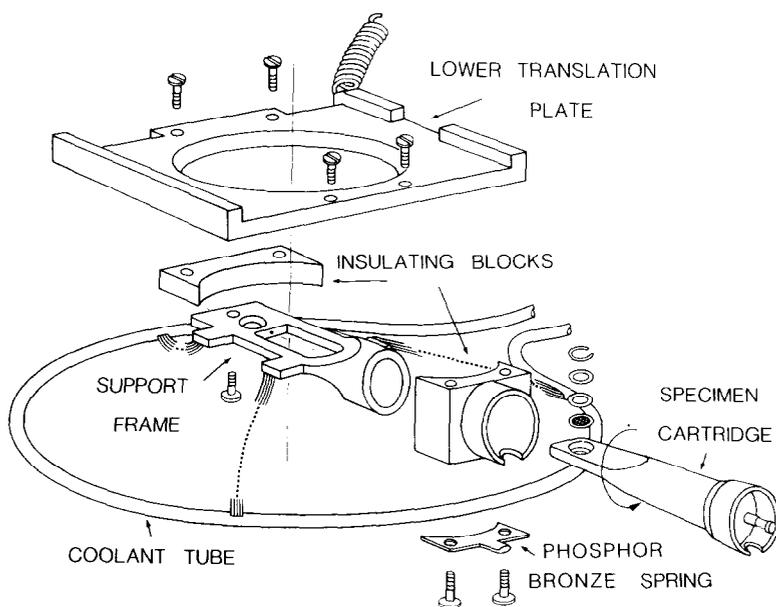
Fig. 1. Cold stage assembly and specimen cartridge (exploded view). This drawing shows only those pieces which have been modified from the standard Philips object stage and specimen cartridge.
